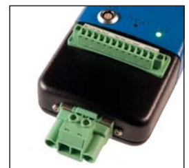
4x DC and 4x AC Inputs 30A socket for switching and rectifier PWM regulation
