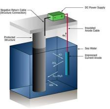
The principal of cathodic protection involves the introduction into the electrical circuit of a metal that is more electro-negative than the existing anodic and cathodic areas.
