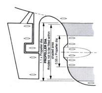
With all stern frame systems, anodes should be positioned to avoid areas of the hull lying directly ahead of the propeller blade tips and in the area within the outer half of the propeller radius. Anodes placed in these positions can cause cavitation and a consequent reduction in the efficiency of the propeller.
